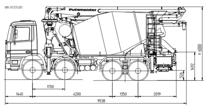
Note: Standard version. Dimensions and weights depend on boom, mixer and chassis.
