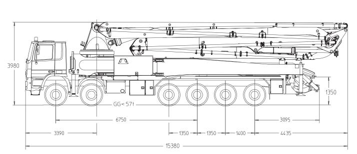
Note: Standard version. Dimensions and weights depend on truck, pump model and equipment. Dimensions in mm, MB-Actros 5554 as example. Realisation on five axle truck possible.
