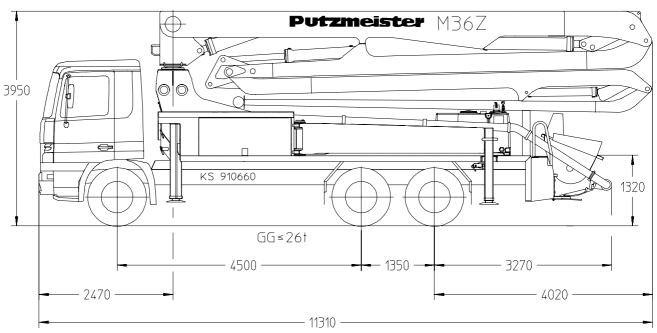
Note: Standard version. Dimensions and weights depend on truck, pump model and equipment. Dimensions in mm, MB-Actros 2632 as example
